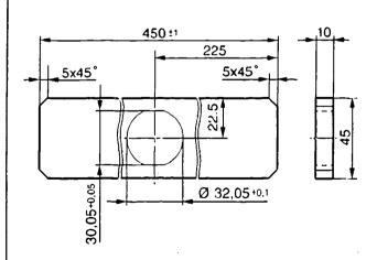
Improvised support for multi-plate clutch for caulking threaded ring
